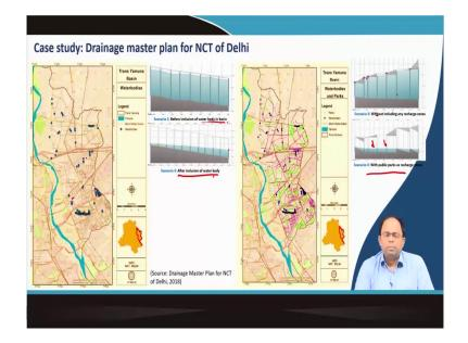
As shown in the image, like in scenario 2 before inclusion of water body in the basin, this was the kind of profile of water in the drains. Whereas, after inclusion of water bodies, the water level in the drains have reduced significantly.
