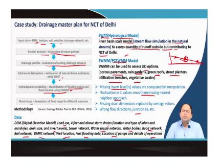
The methodology given in the master plan is discussed. Input data was DEM data, land use data, soil, weather, drainage network data, etc.
