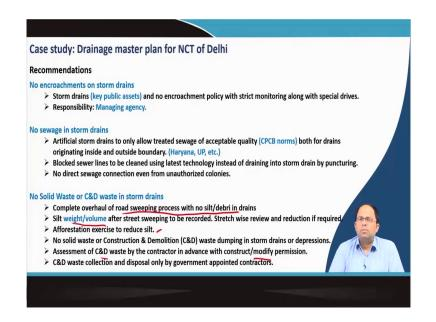
The final recommendations from the drainage plan for NCT of Delhi are provided. There should be no encroachment on storm water drains because storm water drains are key public assets.
