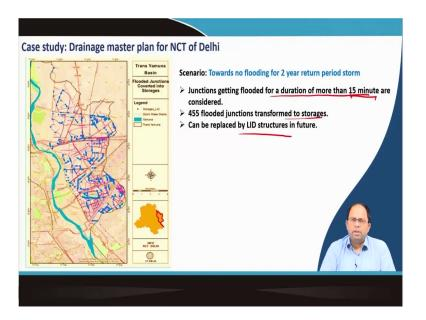
Then towards no flooding for 2 year return period. It was seen that junctions getting flooded for a duration of more than 15 minutes were considered. As shown in the image, 455 junctions were flooded and these were transformed to storages. That means, they were designed to store water. As they store water for only 15 minutes, that is considered as an acceptable solution.
