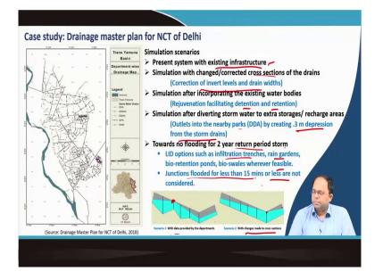
Once the basic estimation was done, then several scenarios were simulated. The first simulated scenario was the present system with existing infrastructure. This represents the simulated sewer section using data provided by the different departments. The computation are done and checked if the flooding is happening. Simulation was done again with changed/ corrected cross sections. Corrections are done in invert levels and drain widths.
