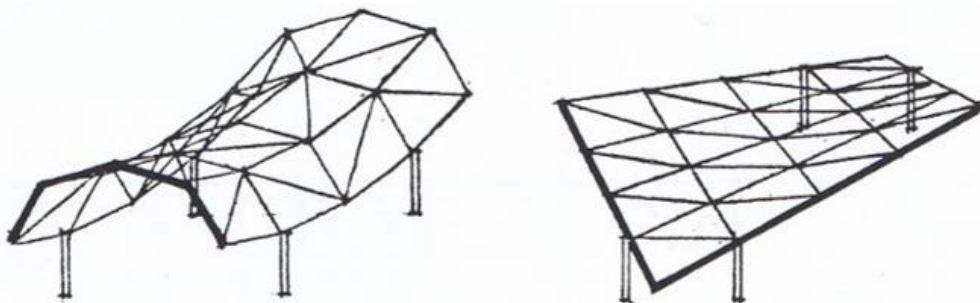
Figure 15 : Saddle Shape System
