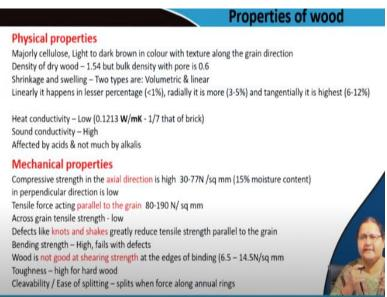
Defects of timber: Moisture reduces the strength particularly on the tension member. We have to be very careful when we are using wood as a tension member in truss, in form of beams, some member spans to ends. You have to remember minimum defect is the better. Wood is not good at shearing strength at the edges, the values are given.
