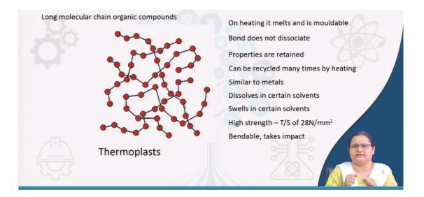
So the properties are getting retained. Hence, even by heating to a certain temperature, you can mould it, reshape it and again reuse it. So this is the beauty of thermoplastics. That means, you can use it n number of times. Hence, it is recyclable. Similar to metals maybe. Metals as I have told it is hundred percent recyclable. Thermoplasts are also recyclable. Now remember thermoplasts are not hundred percent used.
