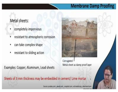
The next item is metal sheets. You can see in this picture that the metal sheet has been corrugated and applied in this particular zone. So this is the wall. This is where the corrugated metal sheet has been inserted when the slab was being cast. This makes it completely impervious, resistant to atmospheric corrosion. Many non-ferrous metals like aluminum, lead and copper are usually taken.
