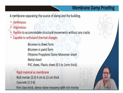
The first method is membrane damp proofing. By membrane we mean a thin member, which will be spaced in between and will not allow the damp or the water or the moisture to percolate inside of a building. So it may be placed between foundation to stop groundwater from trvaelling to the upper part of the superstructure from the substructure.
