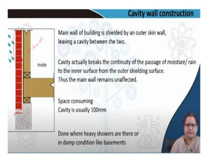
Now we come to the cavity wall construction. What is cavity wall? If you look at the picture, there is a main structure and then the red wall here. This red wall is an additional wall that has been planned and made just in front of the main wall where the outer skin experiences a lot of weather action like rain, or some moist condition. Some of the water can even seep in but will get trapped into this cavity in form of moisture or in form of water.
