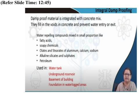
Now we come to the next type of damp proofing which is called integral damp proofing. Integral means integrated with the material. It is usually added in the concrete mix or the mortar mix, when it is a case of plastering. These materials are usually soapy materials. That means it will be repellent to the water. They actually enter into the voids of the concrete and eventually prevent water entry or exit from a system.
