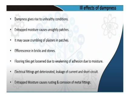
So we can summarize by stating that damp gives rise to unhealthy and unhygienic conditions. But how can we understand that a place is getting damped? The entrapped moisture can give some clue through its unsightly patches. So you can register that a building is experiencing moisture inside it. When such patches start forming you see suddenly a plaster piece comes out and falls.
