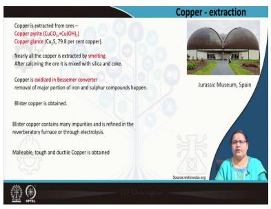
The ore is copper pyrite and copper glance. One is carbonate and the other one is sulfide. High temperature is involved in the smelting process, which is heating at high temperature. Calcite is extracted after calcining the ore and the oxide is formed after putting this first extracted metal into the Bessemer converter. Removal of the major portions of iron, sulfur compounds happen in the Bessemer converter. It is a very similar process where blister copper is obtained.
