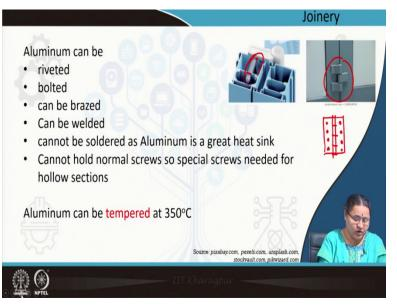
Let us take brief look on the joinery part because as you see doors, windows, etc are being made. Aluminum can be riveted, bolted, brazed and welded. We have gone through all these processes in details. Riveting is a permanent kind of joint. Bolting is temporary as you can unbolt it, but what you cannot do is soldering because aluminum is a great heat sink.
