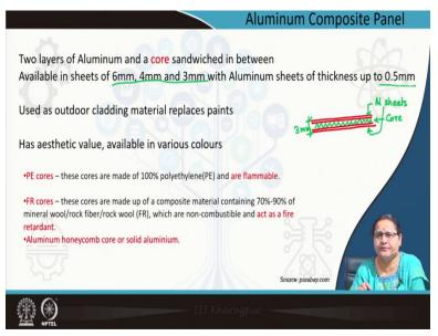
The core is usually sandwiched in between the two aluminum sheets with an overall thickness of as low as 3mm. The standard thickness is of 3 mm, 4 mm and 6 mm. The aluminum sheets are of 0.5 mm in thickness. So, you can understand how thin the sheets are! It is not even a millimeter thick. And the central part is the core, which is either the poly-ethylene (PE) or fiber or rock wool core.
