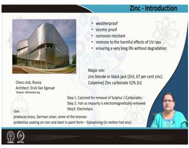
So we come to the next non-ferrous metal which is zinc. It is weatherproof, seismic-proof, corrosion resistant, immune to UV rays, ensures very long life without maintenance. Zinc is mostly used for galvanizing, as you all know. One common example is the Chess Club in Russia but zinc is mostly used for galvanizing across the world. Zinc blende or black jack is one of its ore and calamine or zinc carbonate is its other ore.
