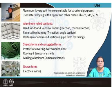
So as I told you, coming to the use of aluminum, it is a very soft. You need to alloy it with copper, zinc, manganese, silicon and nickel. So, different proportions are required and we are not entering into the metallurgy part. We need structural aluminum and for that whatever is suitable, we will get it from the market. Aluminum can also be made from rolled sections; we have extensively discussed rolling of steel the same way aluminum is rolled out.
