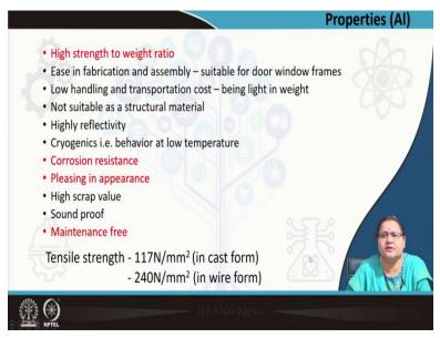
Aluminum exhibits property of non-ferrous metal. It has high strength-to-weight ratio, easy in fabrication and assembly. That is why it is suitable for doors, windows, frameworks, any kind of partitioning frameworks. Being light, it is easy to handle, transport and cost is obviously less. It has a shine i.e. it is highly reflective when light falls on it, but it is not suitable as a structural member.
