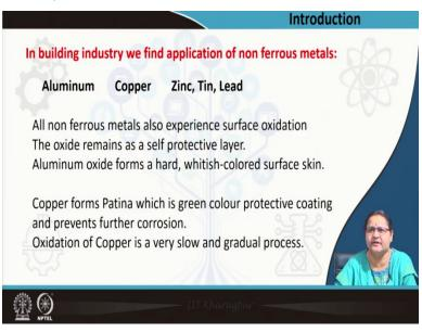
Now, in building, we find aluminum, copper, zinc, lead and tin. All these non-ferrous metals also experience surface oxidation like corrosion of ferrous metals. But in case of ferrous metals, this ferric oxide or rust used to increase in volume and peel out, create pressure and come out and finally expose the next layer. In case of aluminum or copper or zinc, the oxide formation is happening similarly, because they are similar to metals.
