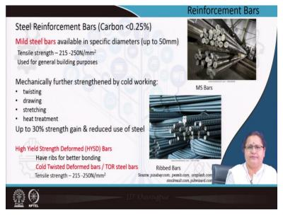
The steel reinforcement bars, which can be seen easily on construction sites. These are mainly rods and bars which are mild steel, having less of carbon. They are usually of different dimension starting from say 2 mm and go upto 50 mm. The available dimensions that are used for construction purposes are 2, 3, 5, 6, 8, 10, 12, 16, 20, 24 and 50 mm. So in your further classes you will understand the calculation part depending on the area of steel required to take the tensile load of any structure.
