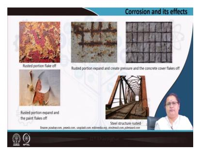
Let us see some pictures to get a visual idea about rusting. You see in the first picture, the layer is flaking off which I have told you just now. See these are the flakes that are the upper layer is coming out and exposing the inner layer. So in the next stage, the inner layer will get corroded or rusted. In the next picture you see here is a pipe, which has been painted. The inner layer is iron which is getting rusted by entry of water vapor or water leakage.
