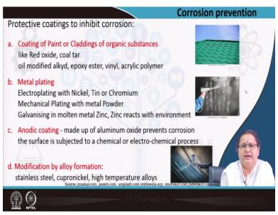
Corrosion can be prevented by coating. You can see the picture of roofing where it is coated. Coating with maybe some red oxide paints and Coal tar (jet black) can be adopted. But if you paint you are getting rid of corrosion only. To get rid of rust flakes, you may apply oil like modified alkyds, epoxy esters, vinyl or acrylic polymers. It is a cladding or putting a dress on top of the iron member. You can also have plating, electroplating with nickel tin or chromium.
