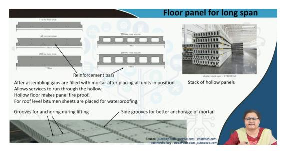
Now what you can see here, similar to the small spans, here also there are grooves to have Anchorage and they are also helping in setting the concrete or mortar which will be added later to make it a single
