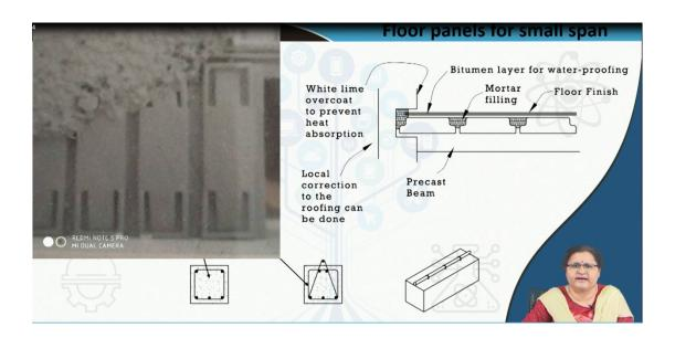
Those have developed for our low-cost housings. It is a fast mechanism you can create three meter by 3 meter rooms one adjacent to the other and you can make the roofing very quickly even if the support is a brick wall. So, now here in this image you can see the mortar is being filled and the gaps are completed. What happens in case of the roof? In case of roof, water may enter through the gaps narrow gaps here and there.
