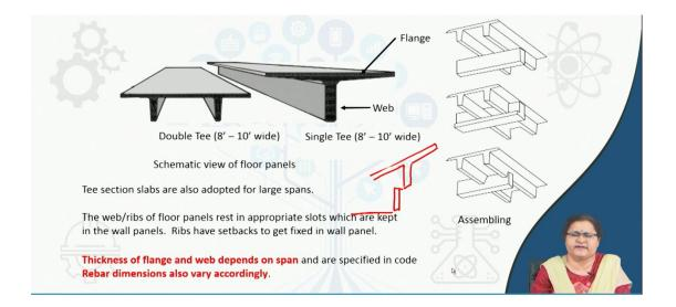
So this is the continuous T which needs to get assembled in a walling system where this will exactly go and match with the wall system. So, one has to be very careful while these are being placed. These are all to be set within its groove if the drawing is perfectly done. So, every instruction should be there when it is being fabricated, when it is being made and when you are coming to site, it is only the job of assembling it in order where the way it was actually placed.
