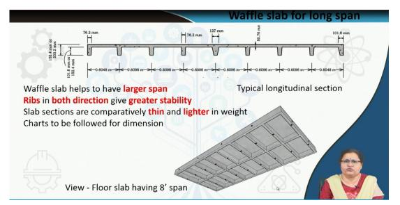
So, charts are there, accordingly the mould is now getting complex, complicated. The reinforcement system inside it is also getting complicated which was not that much difficult in case of the others. So, if such kind of slab is also adopted you can go for such kind of slabs for long span. Let us now go to how these are to be assembled. (refer time: 25:35)
