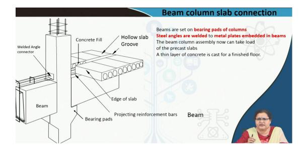
But here the load has to be transferred through the beam into the column. So, that is why the beam cannot be unstable. It has to be set rightly with the column. So, the beam you may check it is sitting on the bearing pad which is a projection in the column. That is also to be designed so that this projection is always left on that particular position. The beam is resting on it further the beam is having welded connection with the column making it a very strong joint.
