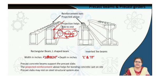
So, you can understand that this dimension, should be matching with the thickness of the slab. Now, in the case of the short span, you had seen the reinforcement is projecting out. Here also you see the reinforcements are projecting out in all the cases. What are they doing? When the slab is placed, here, at the end, these are to be locked, these are to be sealed.
