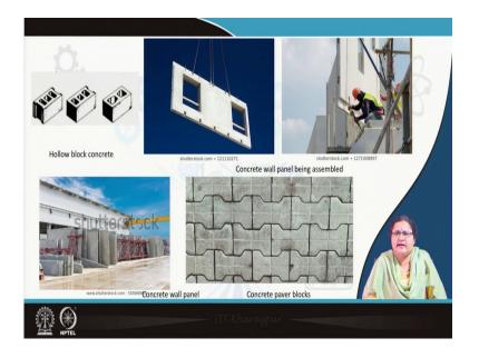
So it is a dry construction entirely. Now, I expose you to some pictures. This hollow block concrete which you see on the first picture here, this resembles more or less brick. But they are larger in size than that of a brick. So, this is cast units special units for when they are connecting one after other they are having you can check here. There are some notches here are some notches. Here is different this is having a flush end.
