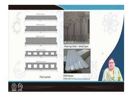
We come to the roofing part. In this picture, you see there are number of sections. We will elaborate on these later. Some are hollow. These are hollow, actually the blank spaces are hollow some may be solid and some dots you can notice. These are all reinforcement showing the marks off it is a schematic picture you can see some units assembled one after the other in this picture showing floor flooring unit small span.
