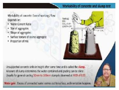
Now let us come to the concept of workability. Workability as I told you, the entire mass of concrete has to move through the dense network of reinforcements. It may be dense at some places like the beams or the columns. It may not be that dense in the slab areas, but yes it has to move through it. So the ease of working or the flow of concrete will depend on the water cement ratio, size of the aggregates.
