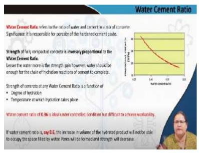
So what is water cement ratio? To put it simply, it is the ratio of the water and the cement in a mix of concrete. The significance is that it is responsible for the porosity of the hardened cement paste. If you remember the gel space ratio, it will increase if you add more of water. So water will affect the strength of concrete because the intrinsic strength of concrete is within the gel.
