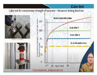
Next is the cube test. This is always done on site before the day of casting. You can see some cubes here where actually with the help of a tamping rod, they have been compacted and the items are left with the material which is being cast on the day, which is a large scale casting. So you have taken samples for testing. Now what to do? On the next day you can remove from the mould.
