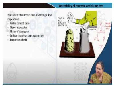
You can see this jar which is initially in its standing position. One side is open where actually you will have to pour this concrete. It has two supports here and it has a fixed dimension. The open end is of 8 inch, the base is of 4 inch and the total height is of 12 inch, that is one feet in height. Now you have to fill it with the unset concrete mix.
