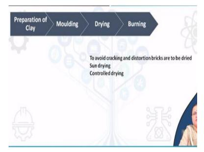
Next is the process of drying. To avoid cracking and distortion of the bricks, you cannot put these wet bricks (or moisture-contained bricks) inside the furnace. So, you have to wait or leave it for sun drying or controlled drying. When you leave it in the sun to dry, it will take some time (one or two days) when the furnace becomes ready for the next batch. You can arrange the bricks around the fire.
