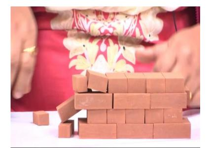
So, in a full brick thick wall, if you keep on arranging like this and follow the same principle, like having bricks in this direction and then again having bricks in a staggered way (as you had seen), you are obviously complying elevation-wise. But if you look the other way, this (see video) entire block can be shifted. Similarly, this entire block can be shifted (separated as a mass). This happened because these two walls are not bound together.
