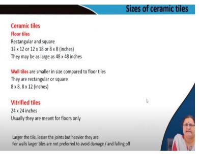
In the market, several sizes of tiles are available. Wall tiles are the smallest. Typical sizes include  $4\times8$ ,  $8\times8$ , and  $8\times12$  (all values in inches). Higher dimensions are not available because there is a chance of falling due to their own weight. Ceramic Floor tiles are usually found in  $8\times8$ ,  $12\times12$ ,  $12\times18$ , or  $18\times18$  (all values in inches). They may sometimes be as large as 48 inches  $\times$  48 inches.
