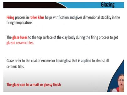
In the firing process, the unfired tiles are put into the roller kiln, where vitrification takes place, and this imparts dimensional stability and vitreousness to the tile. The glaze (top layer) fuses on the surface of the clay body during the firing, and thus, these tiles are called glazed ceramic tiles.
