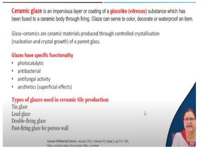
Let us come to the ceramic glaze, which is the glass-like layer or coating that imparts imperviousness to the tile. This layer is fused (not separable) to the tile. It has now mixed with the main body of the compacted clay tile. You may add colors to the tile, similar to the ones mentioned during glass manufacture. That will provide a single uniform coloration to the tile.
