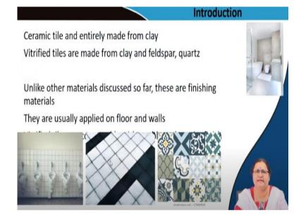
The basic materials used to manufacture ceramic and vitrified tiles are majorly clay and sand. Thus, composition-wise, they are not much different from bricks or even glass. These tiles also contain sand (silica). Ceramic tiles are entirely made of clay and sand. Vitrified tiles are made from clay, feldspar, and quartz.
