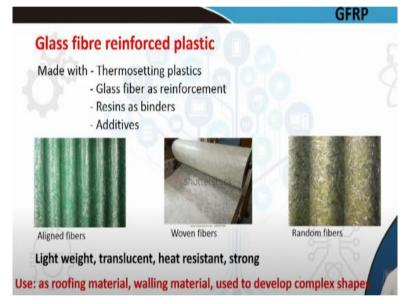
Another product of glass is the Glass Fiber Reinforced Plastic (GFRP) which is made with thermosetting plastic (details will be mentioned later). Glass fibers rovings are used as reinforcement. Resins are the binders here and you can also use additives, coloring agents etc. An image of a GFRP panel is shown. The fibers may be aligned in several ways.
