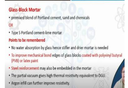
So, in the glass block system, the mortar is a premixed blend of Portland cement, fine sand, and chemicals, or it may be Type-S Portland cement-lime mortar. What is important here is that unlike brick masonry, here there is no absorber for the water component. Glass does not absorb water at all (zero absorption).
