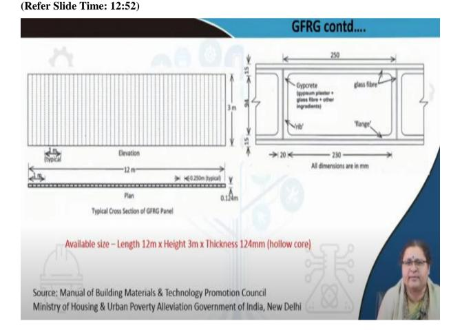
Let us talk about the appearance of a GFRG panel. In this cross-section, you can see hollow portions. Each hollow part is 250 mm in width and has a rib to strengthen the panel. At every 0.25 m (250 mm), there is a rib, which strengthens the wall. These ribs and the ends (flanges) are composed of glass rovings mixed with the gypsum.
