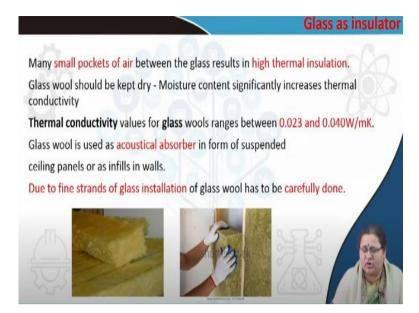
In this picture, you can see how the glass wool looks. Inside it, the entrapped air serves as the layer of insulation. Hence, it is crucial that the internal surface of glass wool is dry. If somehow moisture or water can seep inside, the thermal insulation property is lost. Glass wool also acts as an acoustic absorber.
