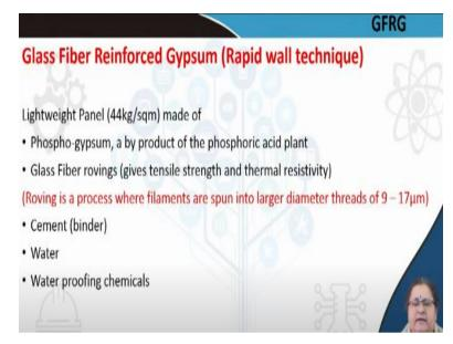
Other than using glass fibers in bat or wool form or as thermal/ acoustic absorbers, we may use them as a reinforcing material in gypsum to produce Glass Fiber Reinforced Gypsum (GFRG). But in this case, the diameter of the thread must be higher (around 9- 17  $\mu$ m). The process where filaments are spun in larger diameters of threads is termed as 'roving'.
