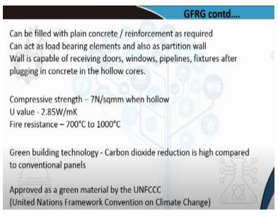
Let us discuss the various characteristics of GFRG. You can get continuous sheets of  $12m \text{ (width)} \times 3 m \text{ (height)} \times 125 \text{ mm (thickness)}$ , having gaps (hollow). Here, in this image, you see a section, and this glass acts as a reinforcement. GFRG is hard, tough, and can withstand impact forces. Within these hollow spaces, you may plug in reinforcement or plain cement concrete, if necessary, to impart more rigidity to the panel.
