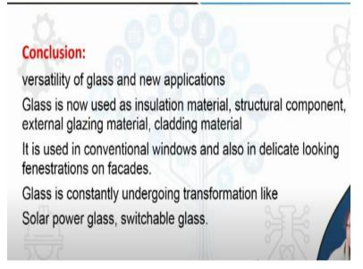
Thus, glass has versatile uses and we are often seeing newer applications. In modern times, glass is being increasingly used as insulation materials, structural components, external glazing material, cladding materials- other than the conventional windows and the delicate-looking fenestrations on the facades.
