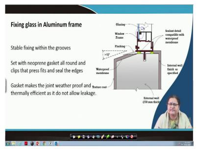
Let us see what happens in aluminium frames. Nowadays, we refrain from using wood frames for environmental reasons. Iron and aluminum frame sections are becoming popular. In the picture (see diagram in video), the glass (blue color) is set within the frame, and a
