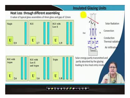
Now, let us move to the next slide. Till now, our discussion had been limited to single glazing, and its U-value was 5.9 (see diagram in slide). Now, when two glass panes (each 4 mm thick) are used, with an air gap (around 12 mm distance) in between, the U-value of the assembly reduces to more than half (becomes 2.7) than in the single glazing. For this third case with a dotted line (see diagram in slide), the U-value has further reduced to 1.9. Both of these are Double glazing units (DGUs).
