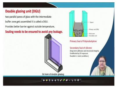
Let us see what happens in double glazing units. Here, the insulated glazing unit (IGU) has two layers, i.e., two parallel glass panes, with an intermediate buffer zone- which may be filled with simply air or argon infill. The quality of sealing of the assembly is essential here.
