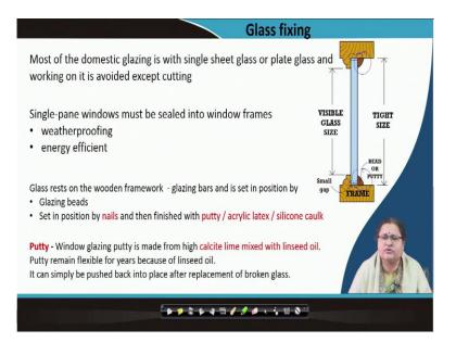
In this slide, you see the diagram of glass fixed on a wooden frame. It may be simply a plate glass, sheet glass, or float glass, and is thus, very fragile. This attachment is done without any drilling or welding. In the wooden frame system (you can see the upper and lower frame in section view), the glass piece is being inserted and fixed in place by putty (see diagram in video).
