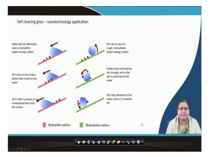
Here is a better picture adapted from the internet. There is a hydrophilic surface, where the dust and dirt are shown by brown-colored granules, and the water droplet is not cleaning them as it trickles down. On the contrary, on a hydrophobic surface, the water droplet actually carries the dust granules and moves down. The force required to carry the dust particles may be sufficient by regular rainfall. But the grease and oil will get 'digested' in the same place.
