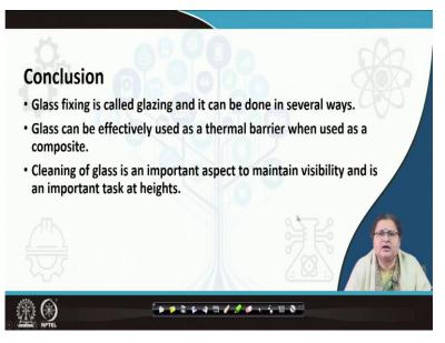
Thus, we conclude that glass can be fixed in various ways. The process of fixing is called 'glazing' (in this context), although the term has another meaning. Glass can be effectively used as a thermal barrier when used as a composite (subsequent layers of glass, air, glass). Cleaning glass is crucial to maintain visibility and is a challenging task at heights.
