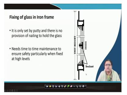
In this next slide, we will talk about the fixing of glass in an iron frame. The sectional details are given here. This is called a Z-section, which forms the frame. You can also see the sealants into which the glass is embedded. Again, here is a T-section.
