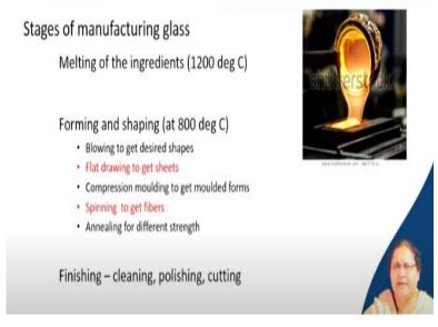
We will now discuss the stages of manufacturing and the ingredients that make this totally transparent material. The three stages of manufacturing are- 'melting', 'forming', and then 'finishing'. 'Melting' implies the melting of the ingredients in their prefixed proportions when mixed with water and heated in a furnace. A lot of bubbles will come out, and gradually, the product converts into a mass, very fluidic in nature.
