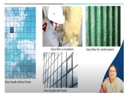
Next, we talk about glass facades with frames. In this picture, glass has been put inside a framing system. The strong frame lines are visible, of which a portion is openable, even though you do not see the actual frame. Glass fibers may also be used as reinforcement in corrugated items (see picture). These fines strands, which you can see inside, are all glass fibers.
