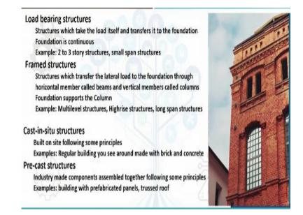
Now again, we come to another aspect. Amongst the permanent structures, we have load-bearing structures where we see a picture on your right-hand side. The load is taken by the entire building. You can see it is made of brick. The building is not so high, and the foundation in such kinds of buildings is a 'continuous' foundation. Also, look at the region at the top of the windows (where usually a concrete beam or a 'lintel' is seen in modern buildings).
