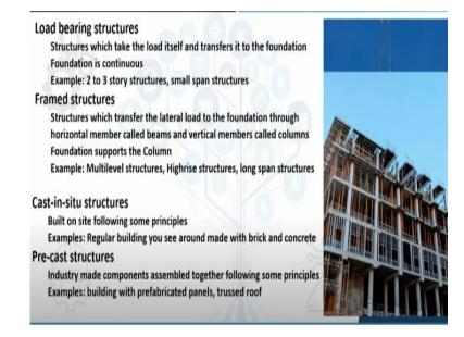
Let us move on to the 'framed' structures, where loads are transferred to the foundation through beams and columns. Here you can see, in the picture, the columns and the beams are visible. Some supporting structures (orange color rods) are present here. These are intended to support the floor because the casting is currently being done, and between these columns and beams, there is no wall at present.
