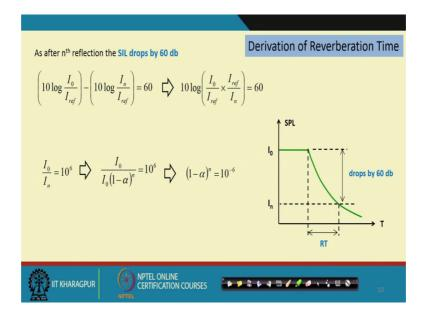
So, what we have do is that our initial energy was I naught which is this and, for I naught this particular sound level, I have measured the what is the sound intensity level and, next after drop of 60 dB it is after n reflection I n. So, this will be the sound intensity level at after sometime after some n reflection and, the difference between this two is nothing, but 60.
