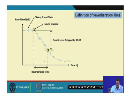
So, let us go to a graph, suppose in x axis I am plotting the time and, y axis I am plotting the decibel level, or the sound level and I start some sound in a particular room and after sometime. I will stop the sound and when I stop the sound, sound is still there because of the multiple reflection and I will get a graph like this.
