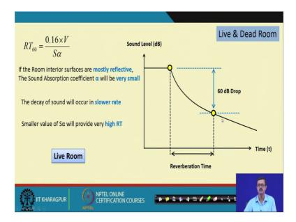
So, those three volume of the hall the frequency of the sound and the absorptive surfaces amount of the absorption coefficient is the three basic parameter to define, or to understand the reverberation time, here I have always written RT 60, if you remember in the last slides also it is sometimes written in the some way the RT is this, but it is better to write RT 60 because by definition RT is 60 dB draw.
