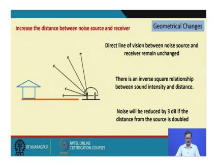
So, what are the geometric changes, the first geometric changes can be occur like direct line of vision can be still here, but we can increase the distance between the noise source and the receiver. So, we push the building little back. And we as for as possible we push the little back.
