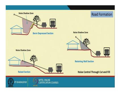
There are another three the sketches. So, in this first top one the top one the noise shadow has been created, but kind of a the berm and the depressed section kind of a thing. So, some of the areas in the, where there is a terrain development or so or maybe there are some area is, where there can be a kind of the design required, some kind of a
