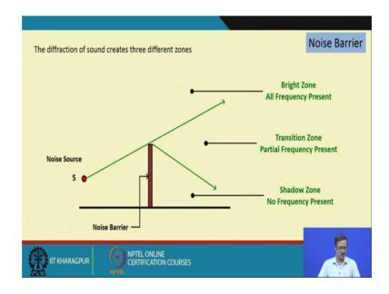
So, from that I can understand that this is the first one, which is flying away from the top of the this noise barrier, which is high frequency. And this is the low frequency is tending back tending towards the ground. It is divide the whole area in the side of the noise source into 3 zone. The first zone this called bright zone, which is above that particular flying line or the line of the side. Why it is bright zone, because all the frequencies are present here.
