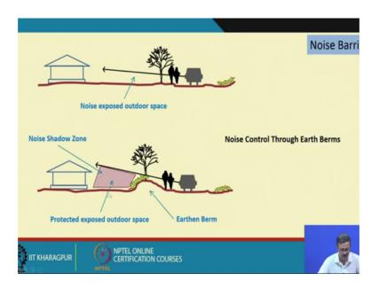
So, there are some control on the barrios. Also so here there maybe expose sound in the first figure, what I have drawn just exposed to the building, noise expose to the building. And the second figure you see there are some barriers, which is earth berm or maybe a kind of a the soft barrier like the trees, and all which can create some kind of a sound shadow zone. In the this is outdoor space can be very enjoyable from, and that will cut of the noise from the sound source also.
