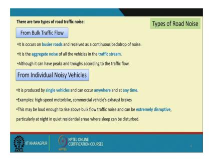
The type of road noise, there are two types of road noise. And one called from the bulk traffic flow, and it is because of the mainstream traffic flow. And it is aggregate noise of a particular busier road, which is have a kind of a continuous noise level also. And there are sometimes there is a peak, and there is a troughs, but it is depend upon normally it is a aggregate noise source.
