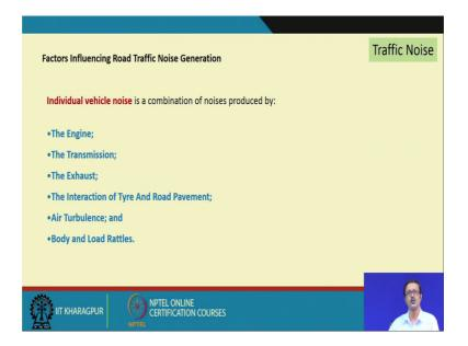
So, there are let us see there in a traffic noise, the individual traffic or individual a automobile has produce noise because of this particular reasons. The engine produce noise; the transmission also produce noise; exhaust that also produce the produce noise; interaction between the tyre and the road pavement that also produce kind of a noise; the air turbulence and also the bodies; and the load rattles and although kind of things are also produces noise.
