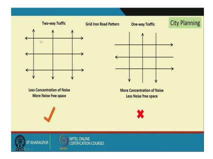
Now, next one suppose you take a grid iron pattern. And in that grid iron pattern, you have two type of traffic scenario. One is a two-way traffic, so from this road. So, this arrow, this is black color arrows are actually indicating the road. And these arrows are indicating the direction. So, here suppose there are the two-way traffic. So, in this road both way traffic can flow.
