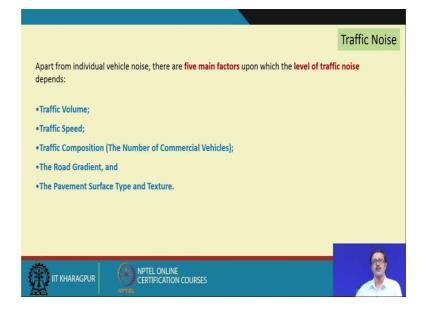
Then there are some five factors has been strategically pointed out in are the Central Pollution Control Board by lot of thorough examination, and the thorough research that the level of the traffic noise is also depend upon this five main factor. The first one is the volume of the traffic. The second one is the speed of the traffic, it is vice versa.
