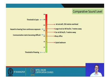
So, let us compare first the noise level. So, this is this particular vertical scale indicates the 0 to 140 dB scale. And as you know, the left hand side about I have put is in that the different subjective feeling for any such noise. The 0 dB is threshold of hearing, and almost to 120 dB is the threshold of pain. Intermediately there are a communication starts become very difficult to win the noise level is just a little above 60.
