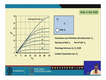
The next one is if there is a whole in the wall. So, this whole will actually try to leak the noise. So, it is depend upon how much amount of noise will be leaked through the hole, suppose it is a very wonderful partition wall made by double leaf and all those. And there is a hole that miss failure total the amount of effort an all to the reduce the noise from
