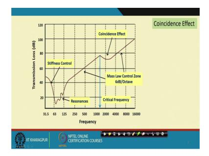
So, a normal frequency TL curve will look like this, the initial in short frequency range there is a lots of dips and undulations. This can be described as there are some kind of a stiffness control and there some kind of a localized resonated resonance is can be happened. So, that is whether is a some undulations.
