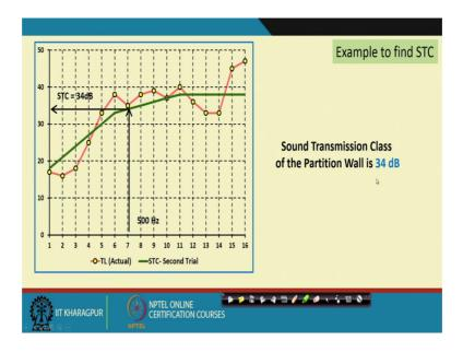
So, 500 line hertz line striking to my this 34 this STC contour, that is give me the STC value this 34 dB that is how I found out this particular transmission sound transmission class of a wall.
