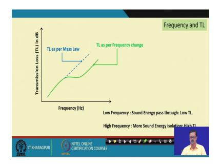
This is follow a kind of a stiff straight line graph kind of a think where we can plot the frequency in the x axis and the sound transmission loss in the y axis. And we can see their transmission loss is something like this through this particular follow this particulars straight line, but in actually in follow this green line where there is a sudden flat the plateau and they again there is a increment.
