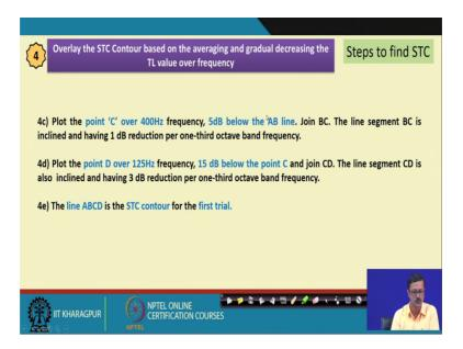
Now, let us go to the point number 4 c, plot the point c over 4000 hertz frequency and 5 dB below A B line.
