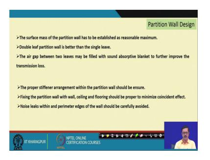
So, I have noted down some of the partition wall significant character the we have to increase the surface mass of the partition wall to established reasonable maximum to get a good amount of TL, these are the some of the partition wall design criteria or the guide lines double leaf partition wall is better than the single leave because there is aircushion in between. So, doubling of the mass is also and happening there is a internal aircushions
