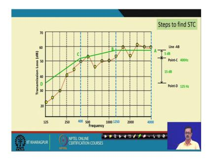
So that means now, you plot a point C over a 4000 frequency line and this will be below B how much below now 5 dB below B. So, you have you see this from 1250 this blue line to this 400 this blue line there are 1 2 3 4 5 gaps. So, the 5 gaps means per octave pa per frequency one - third octave there is a decrease of 1 dB. So, I got the point C the, I will join the line B, C also the line segment B C is inclined and having 1 dB reduction per octave one - third octave.
