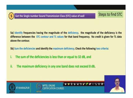
But this is not final you have to see some criteria, it is see a get a single number of this STC we have to find out some of the criteria, what you have to do in the state number 5 a is that, identify the frequency having the magnitude of the deficiency. What is the deficiency? The deficiency is that the difference between the STC contour and the TL value.
