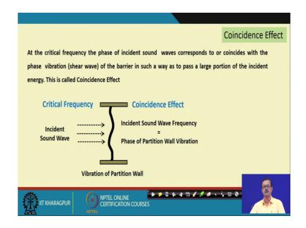
So, this 3 phenomena gives us a kind of a the kind of a understanding that, the even if the frequency if a frequency increases the transmission loss is going to increase, but it is not same for all the range of the frequency some where it is kind of a jerk. And there is again it is follow a particular straight line and this particular phenomena is called coincidence effect.
