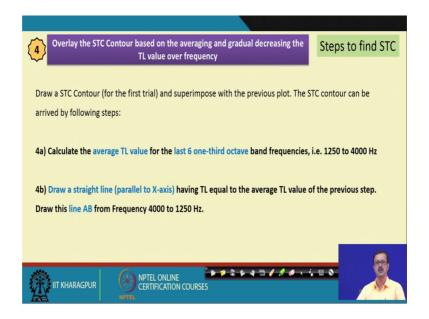
Where I will going to overlay a STC contour on that I will just going to cut off some of the points and try to fix some straight line in a some the method with their some method. What are the method? So, the first in this 4 the state number 4 calculate the average TL value for the last 6 one - third octave that is 1250 to 4000.
