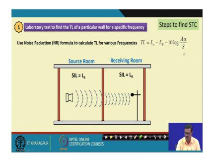
So, what is the first step is that you have to test the partition wall in a laboratory. So, we use that particular formula what we are use in the second lecture, the previous lecture, TL is equal to L S minus L R minus the 10 log alpha into S. So, this is the particular equation and if I have a microphone at the particular receiving room and a loudspeaker in the source room
