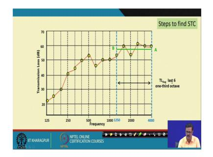
So, what I did is that you have to find out the what are the average of this 1 2 3 4 5 6 this last 6 TL value and find out the what is the average of that and you plot the you plot the line. So, draw a straight line parallel to x axis of that particular and find out this A B line is actually the average of those. So, some points should be above A B, some points should be below A B.
