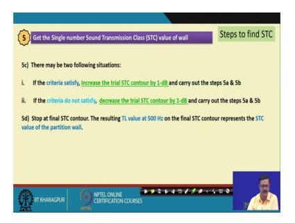
And at the final stage in the 5, 5 c we have to there are 2 situation, if all criteria both the criteria is satisfied a both the criteria satisfied we go to next trail of the STC contour we will increase the trail STC contour by 1 dB. And we will recalculated the recheck the criteria are the step 5 a and 5 b and come again and sometime is criteria does not match with the criteria the actual this deficiency or may not match.
