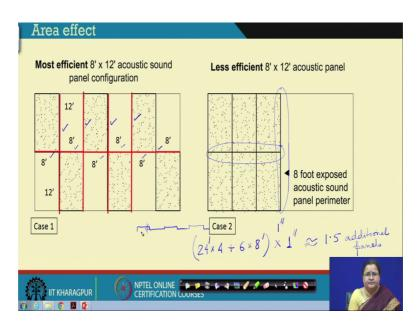
See let us see a ceiling where 8 feet by 12 feet boards 50 percent are 50 percent of the ceiling has to be covered which you see in case 2. So, 6 such boards of 8 feet into 12 feet of absorptive materials are taken in.
