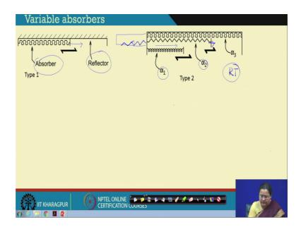
So, let us see; see here in type 1 and type 2 actually there was an absorber here and some portion was reflecting sound, by sliding in another item from this edge. So, this must be stacked inside some place here from which this is actually this is actually sliding out. So, once it is pulled it can cover up this entire area.
