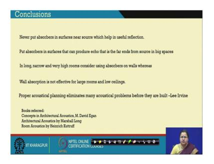
So, the conclusions could be drawn like this we are never to put absorbers in surfaces near source, which help in useful reflection this is summing up of the absorbers. So, we put absorbers in surfaces that can produce echo. So, that echo that is long delayed reflection long delayed reflection of sound, which is particularly at the far ends of big spaces, that is in case of auditoriums concert halls and multipurpose rooms.
