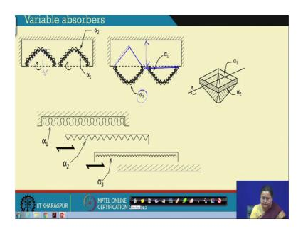
So, here actually you can have these surfaces which have which are pushed inside they can rotate and come down having another absorption coefficient outside. So, you are rotating against a particular rod here, you are rotating it and you can do it alternately you can continue the same way what I told? But these should be there should be enough space to house the rotated portion.
