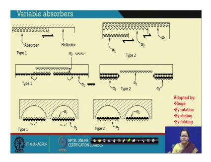
We are adopting different kind of absorbers within the same environment by mechanism by mechanical means that is by rotation, by hinging, by sliding, or by folding. So, this way actually you can keep on changing the internal absorption coefficient, internal total absorption, that is based on the absorption coefficient and you can keep on having different reverberation time for different to suit, different purpose, this is another example.
