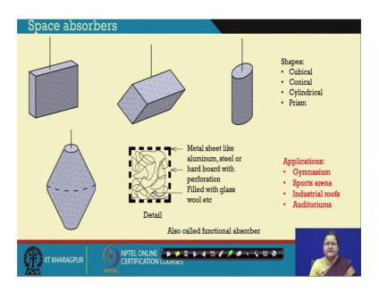
Now, these could be of different forms and what are they actually, they could be cylindrical, they could be conical, they could be double prism, they could be they could be cubical in nature, and these are also called functional absorbers.
