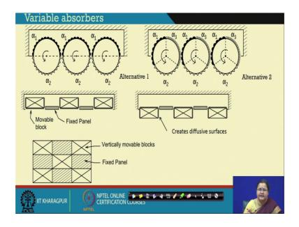
You can actually rotate and have 3 kinds of absorption the first figure shows 2 kind of absorption. So, if you rotate by 180 degree in the first case for the alternative 1, you can get a different alpha 1 coming out. So, if you rotate by 180 degree you have alpha 1 and the alpha 2 enters inside.
