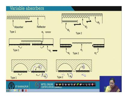
You can have another type, you can have rotating things. See on the upper side it is on the, which is not exposed is alpha 1 and outside you have alpha 2. In the first case it was alpha 1 outside and alpha 2 inside.
