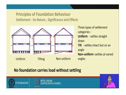
Now, one thing we must understand when we are talking about the substructure is the principle of foundation behavior in a nutshell. Now, the if there is a settlement which is generally manifested in terms of crack, if there is a settlement we have to understand what is the nature and significance and effects of the settlement. So, generally there are three types of settlement broadly the three types of category; one is the uniform that
