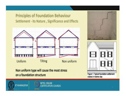
And also in that that non uniform settlement what we are talking about it cause the most stress on a foundation structure. Even in tilting also there can be the cracks and other thing. Uniform sometimes is a horizontal crack, but if it is no longer continuing is probably is not problematic until and unless it settle. So, much that there is a from the surrounding ground there is a lot of problem of the water, but anyway the most important or most dangerous should say the non-uniform type.
