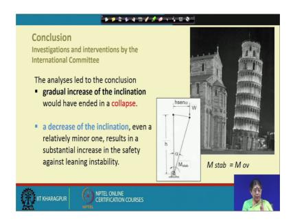
So, analysis lead to the conclusion that a gradual increase in the inclination would have ended in a collapse a decrease of the inclination even a relatively minor one result in a substantial increase in the safety against the leaning instability this is very I mean important realisation which happened because the studying the behaviour of the tower and equating with that the concept of the leaning instability.
