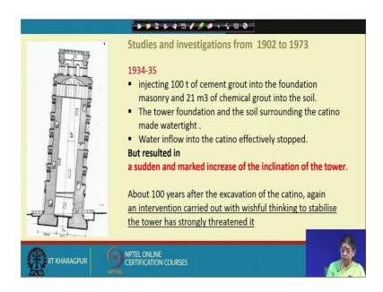
So, because of that hundred tons cement grout which I mentioned earlier and the chemical grout was done. So, it is basically consolidation which happened to in the ground.
