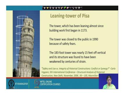
Now, as we can see here that I mean the tilt is quite a lot the tower which has been leaning almost since the billing work first began in 7; 1173 and the tower was closed to the public in 1990 because of the safety fears and the 183 foot tower was nearly 15 feet off vertical and its structure was found to have weakened by centuries of strain.
