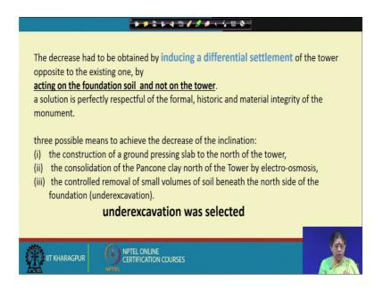
This the its quite simple it use to induce a differential settlement of the tower to take it to the opposite direction and how do you take this differential settlement acting on the foundation soil and not on the tower it really did not need any intervention of the tower itself, the solution is perfectly respective respectful of the formal historic and material integrity of the monument. So, this was realise and what are the three possible means.
