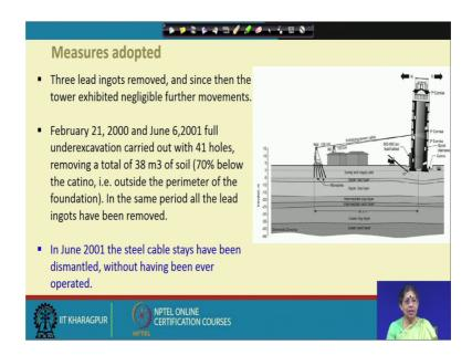
So, this is some of the cases as you can see the stages there which sort of holding that in case something happened there were the two stage of two sides and you can see the soil structure there and the lead ingots were gradually remove and this is how the drilling was happening to take a excavative soil.
