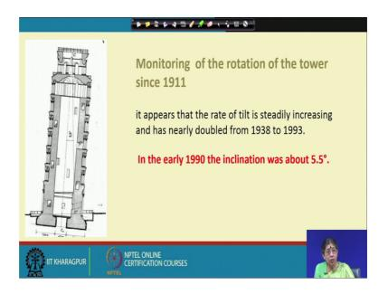
It appears that the rate of tilt is steadily increasing as not nearly double from 1938 to 1930; 1993. So, in the early 1990, the inclination was about 5.5 degree quite a lot.
