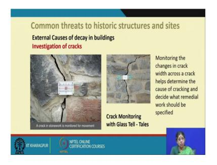
As I say that the crack has to be monitor one has to understand, whether it is night crack or day crack, this is what we say is monitoring of the crack through a glass tell tales where it also this type of little improved version of glass tell tale is shows that whether
