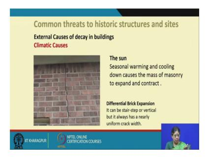
The example of a break wall; where we see the differential brick expansion it can be stair step or vertical, but it always has a nearly uniform crack width. So, these sort of a thumb rule to understand the crack what is the pattern of the crack the location of the crack and other things.
