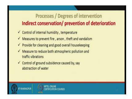
Control of water again is in various form, is very important to understand, because in many cases the control of ground subsidence caused by let us say abstraction of water, because many structures could have sort of been there were initially there was no human settlement, may be outside and because of the increase in the density and the extraction of water from the ground, with many times causes a change in the substrate water level and which may cause a problem later on.
