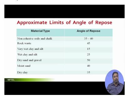
Here, I will just keep this slide for few seconds. And just to give an idea, the different materials which are used for the landform works are of this kind: non-cohesive soils or chalks, rock waste, very wet clay and silt, wet clay and slit, dry sand and gravel, moist sand and dry clay. And they have their standard angle of repose which are less variable. So, I am keeping this particular slide
