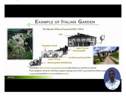
Let us look at the section as we found in the references. We have the villa, we have the caretaker house. And this level changes were structurally made stable with the buttresses of the buttressed walls, stone walls. Okay? So this is the upper terrace, then the lower terrace. These are retaining walls. And priority was landscape site that they have created.
