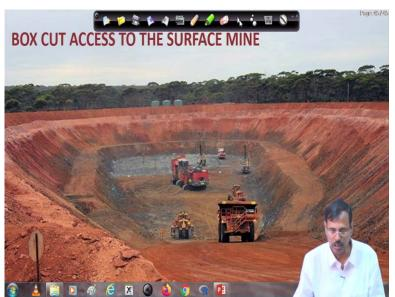
This is a photograph of the box cut. You can see the excavation is already made. This is the boxes already made at this place. You can see this portion. We are making it ready for the blasting here; the excavator is working here, the dumper is moving this is the dozers. So, all these machines are working here. So, sufficient space is created at this position. But simultaneously, as the machines are lowered, machines are working here.
