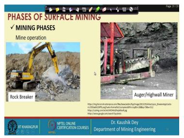
This is the rock breaker and this is the highwall minor which are the commonly used in a surface mine.
