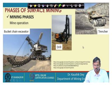
This is a bucket chain excavator, this is drill machine, this is a typical surface miner called trencher.
