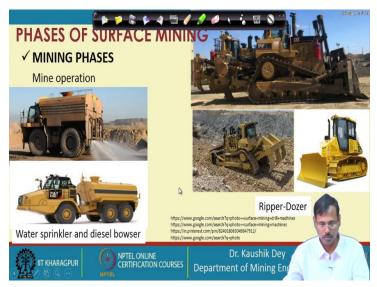
This is dust suppressant so water sprinkler, so that the dust suppressant can be made. This is the diesel bowser, which will give the mine fuel. This is a ripper-dozer. This is only a dozer.
