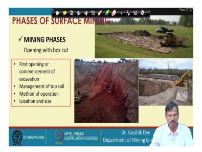
Now, you have to start operating the mine. The mining is carried out with the box cut operation. You can see the first mining is carried out here. You have to take out this topsoil, you have to restore this topsoil, then gradually you have to open up this pit. So, this is called box cut. And all these are basically considered in box cut. Then, management of topsoil, method of operation, location and size you have to; this is box cut is basically the commencement of the actual mining.
