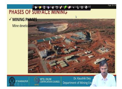
Now, this is a picture of the actual mine site. You can see this is the mine and this is the infrastructures these are the offices and housings, and this is the processing plant, this is the tailing topsoil management, this is the tailing management and this is the mining is carried out here. So, you can see all these infrastructures are developed like this, this is the access roads.
