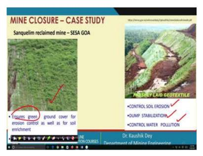
So, you can see the how the geotextile is used for ensuring the greens, controlling the erosion, so soil erosion, dump stabilization, and water pollution is controlled.
