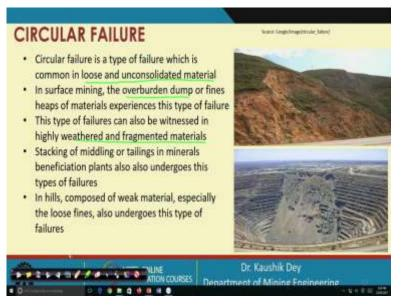
Now, these are some of the examples of the circular failure occurred in the mine. You can see the quantity of material, the quantity of material slided down here is very very high and that's why the rehandling cost any of machines which are under operations are already damaged because of these, so the consequences are very very high in this case and that is why it is very very important to control this circular failure.
