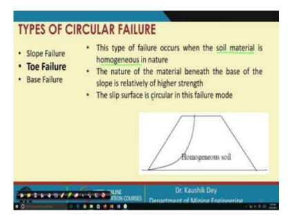
This when the Arc is meeting with the toe, this is called toe failure. This is occurred when this part, this rock is very competent and this is a homogeneous loose material. Then, this type of failure occurs because this homogeneous loose material on any condition, the this one the destabilizing force is becoming more than the stabilizing force, this material slide down like this, so this is often occurs with increase in this weight because of the moisture content or the saturation.
