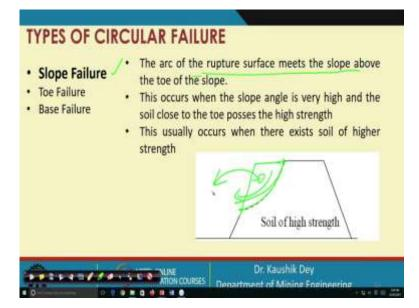
Circular failure is categorised in 3 ways, one is slope failure. In slope failure is the bench is like this, a part of this bench is fall down and you can see this Arc is formed this bench is fall down like or slide down in a form of Arc here, that is called slope failure. This Arc of rupture meets the slope, so this is formed and this made the slope, so this will become delighted and moved out, so this is the slope failure.
