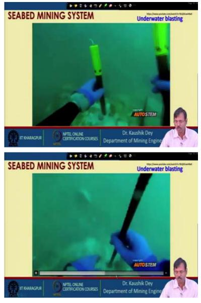
If the electrical detonators are used, then also it is properly sealed so that there cannot be any charge loss. Now the best part is that it need not to be stemmed, it is auto stemmed due to the height of the water column the stemming is already achieved in the hole. So after this blasting you can see the cracks here, how the drilling and blasting is carried out let me show you in this place.
