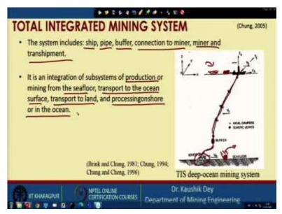
And now, let us go into the generalized technology for which everyone is thinking of so, yet not we are confirmed that this technology, how far it will be viable but this is the proposed system. In the proposed system, our requirement is ship, pipe, buffer, connection to miner, miner and transshipment, so this is the requirement. What is in a nutshell, the system is we should have a ship, the ship must have the attachment of a number of transportation ship.
