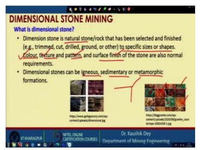
So, dimensional stone is basically a natural stone or rock that has been selected and finished and to specific sizes and shapes and in generally used for the home furnishing or similar uses. The colour texture, pattern and surface finish of the stones are very important considering its price.
