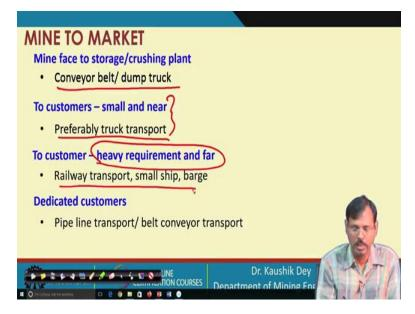
As we have seen, the most general mining face to storage transportation system is conveyor belt or dump trucks these are the most popular system and from this crushing plant or storage to the customer is mostly either by the trucks transport, if it is small and nearby and if it is large scale requirement and away, then it is railway transport.
