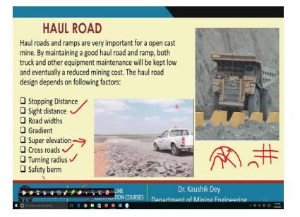
A road width is that whether we are having sufficient road width to move a number of vehicles. That means, it is the one lane vehicle or two lane vehicles, how many vehicles can be allowed that is the road width. Narrow road is basically problematic, then the vehicles have to move cautiously in narrow roads. Gradient is the tip inclination, this is the inclination on which the vehicle is moving.
