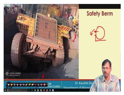
And improper safety dump height may result into accident like this. So, this is the accident you can see, the dumper fall down into the crushing plant, while it is trying to unload its dump into
