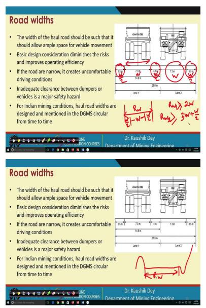
Now, this is the road width, basically if this is the seven points, this is one example taken from the tenant books 7.3 meter, so, around 3 and a half meter is kept here, 4 meter is kept here again this is. So, in general it is considered like this. If this is the available width, then we have to provide, this is the dumper width. And in both sight half of the dumper width should be kept of the clearance.
