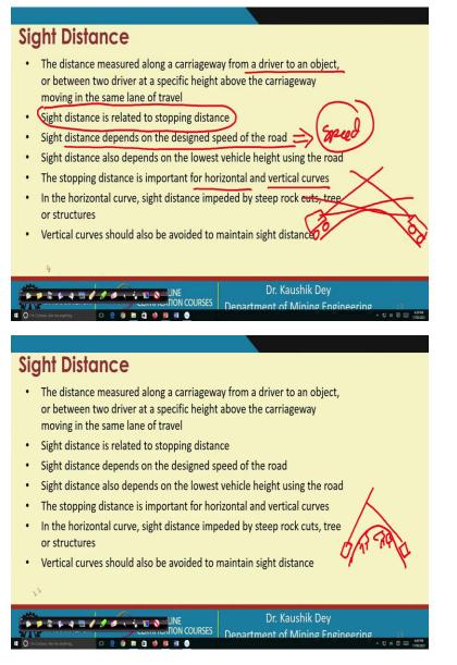
Sight distance is basically the visibility, from a driver to an object. In the very beginning, we have shown a video, which is basically showing the eye view of the driver, how the driver is able to see from his seat about the road. So, they are the visibility what in that video has been seen, is the visibility of the driver or the operator of the machine. And that is why, this sight distance is related to the stopping distance.
