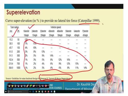
So, these are the different super elevation curve, a super elevation provided as per this reference. So, this is the turning radius and these are the speed. And this is the percentage of super elevation, this guideline is provided and this is the considering the tyre force as per the caterpillar.
