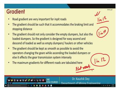
Now, this gradient is very important. And as per the rule in most of the Indian mines, this gradient is maintained at least 1 in 12. In general, more gradient than this is not allowed. So, this 1 in 12 let me write once again is in general maintained. And for a very short distance, one may go for 1 in 10 also, but in general in surface mines, 1 in 12 is popularly maintained, considered as the good. But, as much as flat roads are, flat roads are basically opted for.
