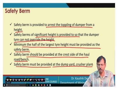
And the final one is the safety berm. Safety berm is provided to arrest the toppling of the dumpers from a height. Safety berm should be of significant height. And so, that the dumper tyre cannot override the height, minimum half of the largest tyre height should be provided as the safety berm. Safety berms should be provided at the crest side of the haul road. And safety berm must be provided at the dump yard and crusher plant also.
