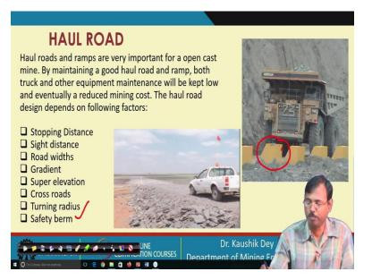
And finally, the safety berm which is, this is the safety berm which is not allowing the dumpers to topple down from this. So, this is also another important aspect to be maintained in the safety consideration of a haul road.
