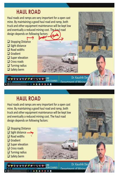
So, basically if we are discussing about the safety, in that case, we have to look into the stopping distance. We have to look into the sight distance, we have to look into the road width, gradient of the road, super elevation, crossroads, turning radius and safety berm. These are the few important aspects of a haul road which is very important. And that is basically required to be maintained for avoiding any accident in the outdoors. Now let us look into this one by one.
