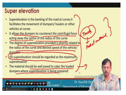
Super elevation is in general provided for the banking of the road at the curves. It allows the vehicle to counteract the centrifugal force acting away from the center of the radius of the curve. The degree of super elevation provided is directly related to the radius of the curve and the speed of the vehicle. In general, a 5 percent super elevation is provided and can be considered as the maximum. And material should be well paved to cater the load.
