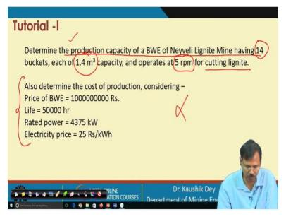
So, now let us go for solving some problem related to this. So, our first problem is that determine the production capacity of a bucket wheel excavator of Neyveli Lignite Mine fitted with a 14 number of buckets as the capacity of each bucket is 1.4 meter cube and it is having the rpm of 5, while cutting the lignite. Rest part we are not considering at this, currently we have to find out the production capacity.
