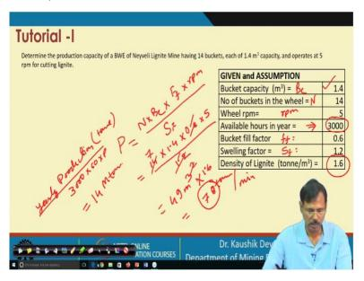
So, for this let us find out we are already given the bucket capacity is given. So,  $B_c$  is given number of when buckets in the wheel is given, so N is given, rpm is given, 5. We have assumed this is the available hours in the year. Bucket fill factor is given. Swelling factor is given and we have assumed the density of the lignite is 1.6 per meter cube. So, the production
