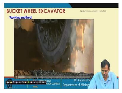
So, in this class we will calculate the performance of bucket wheel excavator, but before that let us look once again how the bucket wheel excavator works. Then it is easier for us, you can see the bucket wheel excavator is having a number of buckets fitted with these buckets are these buckets are cutting the material and as it is cutting it is allowing the material to coming to the conveyor of the cutting boom.
