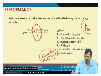
Now if the bucket is not, say, cell less type or semi cell less type, then bucket capacity calculation is difficult. So basically, we can consider this part, this  $B_c$  into  $F_f$  into is basically the excavation of power byte. So, this is the excavation, when a bucket is trucking the face is trucking the face the material dislodged and coming into this the quantity of that material is basically this one.
