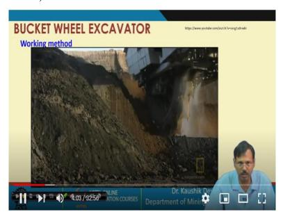
So this is in a nutshell, the bucket will excavator is working and as the bucket is trucking with the face wall, as the bucket is trucking with the phase wall, the rock is basically coming into the or ill being filled disclosed and filled the bucket of the bucket wheel excavator and after entering the material into the bucket wheel excavator, the material is discharged to the conveyor of the discharge cutting boom.
