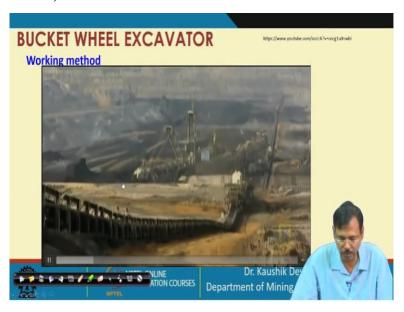
This conveyor is taking the material and allowing that material to come to the discharge boom and discharge boom is discharging the material to a shiftable belt conveyor and the shiftable belt conveyor is transferring that material. (Refer Slide Time: 3:43)
