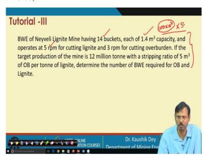
Now let us look into the third topic, that is, what is the capital requirement for opening a mine? Suppose we are operating or we try to open a mine like Neyveli Lignite mine and we would like to have the same model of bucket wheel excavator, which is having a 14 buckets, 1.4 meter bucket capacity, 5 rpm cutting in the lignite.
