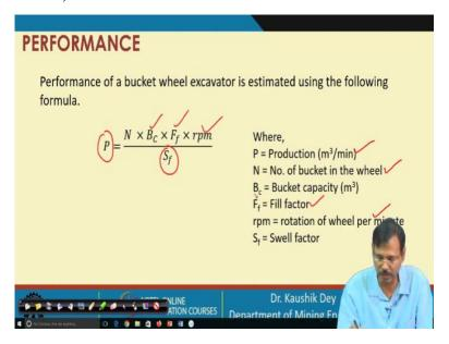
So, this is in a nutshell the excavator is bucket excavator is working. Now let us look how we can expect the performance of the bucket excavator as the bucket wheel excavator is fitted with a number of bucket, the performance can be estimated like this, if the number of buckets N is the number of buckets in the well, P is the performance production meter cube per
