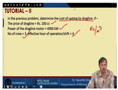
Now, let us look into the second problem. In the first problem itself, we are using that one and we have to determine the casting cost by the dragline. If the price of the dragline is given, power of the dragline is given 4000 kilowatt, number of crew required to operate the dragline is 3,
