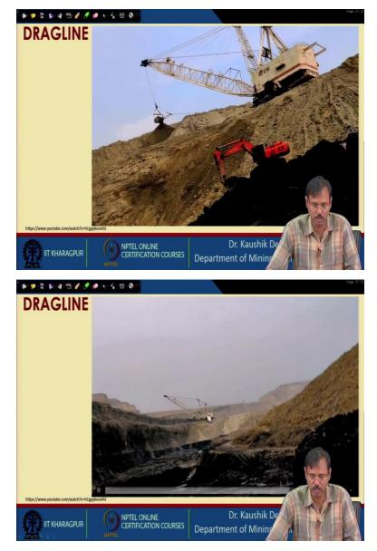
So, once again let us look into this photograph how the dragline is working that is a simple side casting. So, we can understand that this dragline is working and you can see this dragline is in general having a large cycle time. So, two to three minutes, four minutes are taken by the dragline for its one cycle of operation. And we understand that dragline is a walking type of dragline. So, its movement is also very difficult.
