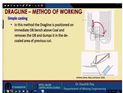
And the side casting we have seen the material is moved, taken from this site and after that the material is taken at, bucket is filled at this position then the boom is swing and it is discharging at this position. So, the whole cycle is taking some time.
