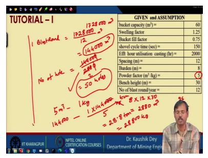
So, dragline capacity is 1728 meter cube. So in one blast round we have to handle 1728000 divided by 12 meter cube. So this is 1, so this is in 1 blast round. And we are having burden of 8 meter, spacing of 12 meter, bench height of 30 meter. So in one blast, we can take this much of material. So this is 2880 meter cube, we can get from one blast. So, the number of hole required in one blast round required in one blast round. So, this is 50 holes.
