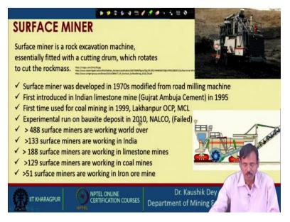
So, surface miner was developed, in a nutshell you can say surface miner is a rock excavation machine essentially fitted with a cutting drum which rotates to cut the rock mass. This is the generalized definition of the surface miner and if you look into the history surface miner was developed in 1970s and originally modified from a road milling machine.
