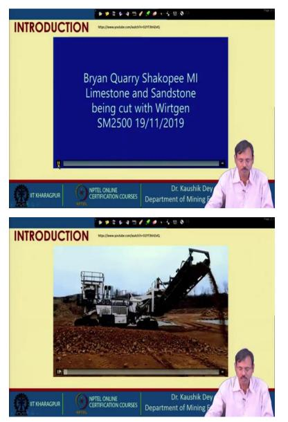
But before going into the details let us just look what is surface miner in this video. This is a video of a query and this machine is called surface miner which you can see as a 4-crawler mounted machine and having a discharge boom, which discharge the cut material and after cutting the material is being discharged. So, there are n number of variations possible with this system and you can see this is a very good-sized material is being excavated and that is being dumped in a row.
