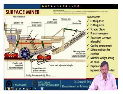
Now, let us look into the detail of the machine. This is details about a particular machine where the cutting drum is placed between the front crawler and the rear crawler or maybe the vice versa also. The cutting drum is operating in up cutting direction, so the drum is rotating. The drum is rotating in this direction, it is cutting in upward direction and material is moving like this. There is a scraper plate. This is a scrapper plate, which is placed behind the cutting drum.
