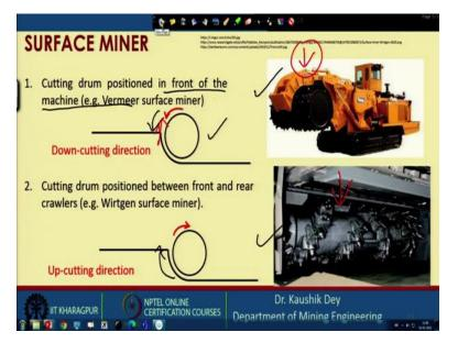
So, surface miner can be broadly classified in two ways; one is that the cutting drum is positioned in front of the machine. So, this is the cutting drum positioned in front of the machine and this is allowing the rotation of the cutting drum like this, this is the allowing rotation and second type is that cutting drum positioned between the front and rear crawler. This is down cutting; this is up cutting and both can be reversed also. Depending on the type of application, this can be made.
