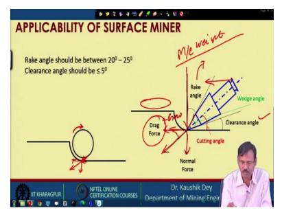
Now, this is the mechanics behind the surface miner. If this is the cutting tip which is basically acting at this place, acting at this place, then if this is the cutting tip, this is the clearance angle,
