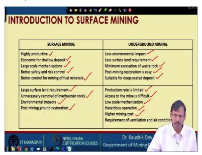
Now, in a nutshell, let us look into the features of the surface and underground mines. Surface mines are highly productive. The economic, the surface mines are economical also for the shallow deposit. The large scale mechanization is possible. There is no restriction on the dimension. And because of the better visibility better communication, the safety and risk control is better.
