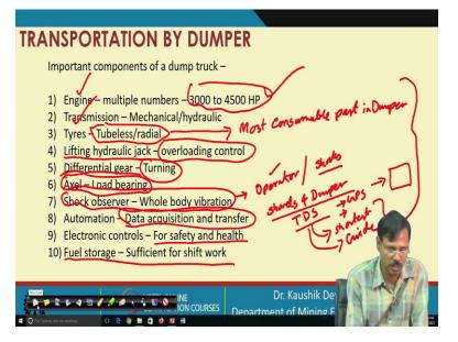
Now, in general, if we are looking at this, the important components of a dump truck can be considered as the engine is very important. In general, this is the capacity of the engine we use for large-size dumpers. Transmission is very, very important, tyres are also important because this is one of the most consumable parts in the dumper and that is why this tyre life, tyre price is very very important on the selection of dumper.
