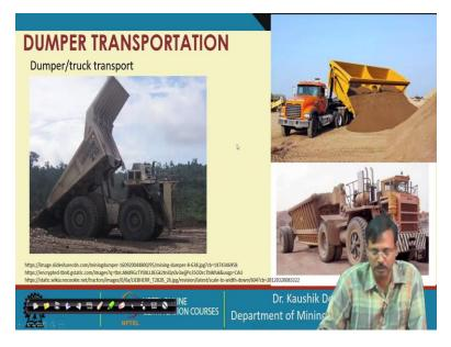
So, we have already discussed that dumpers have a dumping system, either it is a rear dumping system, or it is a side damping system, or it is a bottom discharge type dumper. The damper we have seen in the larger, as the largest dumper which can take 496 ton of material at one go that can, that is having a rear dumping system in the, in that dump.
