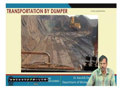
And this is one empty travel return after dumping the dumper. So, after dumping the dumper is returned to the shovel. So, this is depending on the distance and the speed at which the dumper is moving. Generally, most of the dumpers are having high speeds close to 50 to 60 kilometers per hour. But in general, the mining roads are haul roads are made of loose materials.
