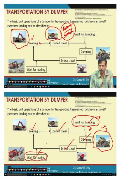
Now, if we are looking at the unit operations to be carried out by the dumper, then we can see dumpers are basically operating like this, first, it has to take the load from the shovel. So, the dumper has to come report to the shovel, shovel will load into this dumper. Now, for loading a dumper, we have seen in the video shovel has to give a number of bucket-filled material to the dumper. So, for loading each bucket it is taking some time.
