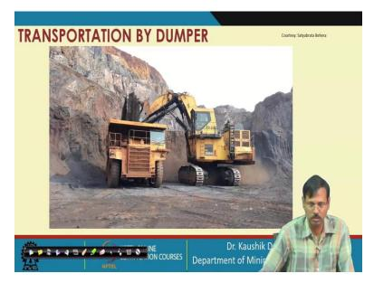
So, now you can see one first operation which is the loading operation of one dumper. So, this is the loading person, this is one of the iron ore mines, this is the shovel, this shovel is taking the load and it is rotating and dumping the material on the dumper. So, see already the second dumper has come from where this camera is basically recording this one. So, the second dumper has already come, but this is under waiting now.
