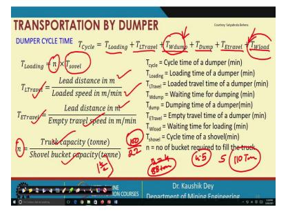
So, now we can describe the time cycle of a dumper as the loading time, loaded travel time, wait for dumping, dumping time, empty travel time, and wait for loading time, among this wait for dumping and wait for loading are unwanted and that is why those are not considered as the in the time cycle. Because our optimization requirement is that we would like to reduce this to as minimum as possible.
