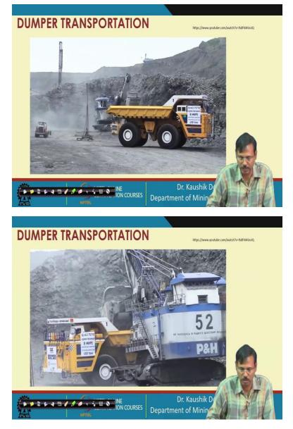
Now, let us look into the operation of the largest dumper in the world. So, the YouTube citation is given here, this is the largest dumper which can have a carrying capacity of 496 tonnes, and it is in general rated that this dumper is used for 450 tonnes of material can be handled at one time and did not consider some of that this dumper is used. See, you can see other dumpers are also available in a close range of 400 tonnes, and this is a huge shovel used for loading the dumper.
