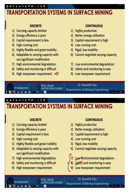
This is having high environmental degradation mostly diesel operated on the movement of the dumper on a haul road it is generating dust, it sometimes often it is budging the horn that is also creating noise pollutions. And this is also the problem with the safety and monitoring is difficult as the dumpers are moving it is not a rigid system moving flexibly or driver skill is essentially required.
