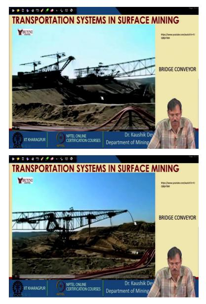
So, this is intermitted discharging system so, that the bench can be extended on this side also. So, this type of transporting system gives us the facility to go for the highly productive mines, and with the highly productive mines, you can go for deep surface mining. In fact, using this continuous excavation system only some of the German coal mines are operating at 500-meter depth also in the Surface Mining system. So, this is more or less the end of this lecture. Thank you.
