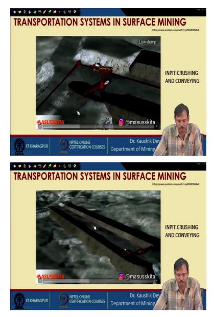
So, this is the way this is carried out where the first after the blasting the material is taken and then the material is taken into the crusher it is a reduced in the site and then that size material is conveyed. So, this is the in pit crushing and conveying system which is used for the transferring of the material. This is the discharging system of the conveyor, where the spreader is used for constructing the dumps.
