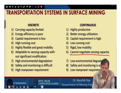
Now, if you compare this discrete and continuous system of transportation, the discrete system is carrying a smaller unit with limited capacity, but this is highly productive. Energy Efficiency is extremely poor for the discrete system especially for the dumper transport system, but it is having better energy utilization. If you look into this, we will find out suppose the dumper is having to say the capacity of 4050 tonnes.
