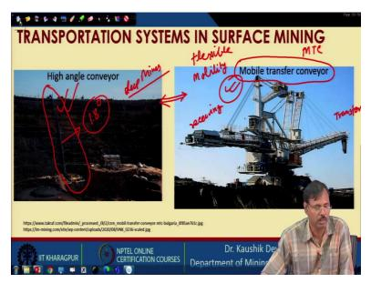
And this is a high-angle conveyor where the material is transported at an angle higher than 18 degrees up to 18 degrees. The conveyor is the normal conveyor, which is practiced and above 18-degree high angle converse is sometimes used it is sandwich belt convert sometimes it is different other types of conveyors are also available. So, this is the high-angle conveyor system and the mobile transport conveyor system.
