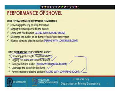
So, to analyze the performance of a shovel, we have to understand the unit operations carried out by shovel every time it loads a bucket. So, you can see when this excavator is just shovel is operating as excavator cum loader so, it is excavating the blasted mark and loading that to your transporting system say dumper in this case. So, it needs to first go for crowding or gathering to form a hap.
