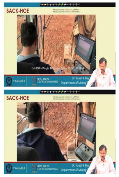
So, this is another operation of this one, you can see CAT 6040, 22-meter cube bucket is used, which is having 2000 hp mod the engine, and this is having a very good look, because this video is taken from the operator's cabin.
