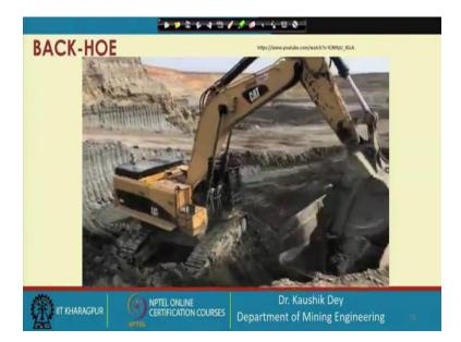
So, in the other side also this is the second dumper, which is placed and here it is very easily visible how the loading is made to the inside the bucket. Now, the bucket is released by rotating the bucket in the upward, opposite direction. So, in the dipper shovel, you are having a door, which is released behind the bucket from which the material is allowed to discharge, but in this case your bucket material is discharged from the mouth of the bucket itself.
