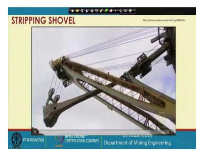
So, let us look into one first video of a stripping shovel and how a stripping shovel works. So, you can see this is the stripping shovel, which is taking the material from this bench, and then in the opposite direction, the overburden dump is there. It is dumping the material onto the overburden dump. So, it is taking the blasted material from this side and dumping it on the other side.
