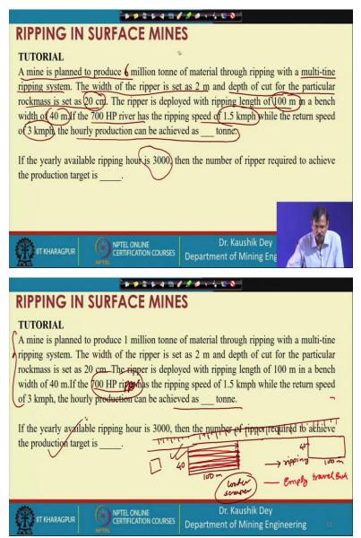
Now, in consideration of this, let us see a problem. The problem is we have to find out the performance of a ripper and consider a mine plan to produce; I think this is 6 million probably, 6 million tons of material through ripping with multi tine ripping system. The width of the ripper is set as 2 meters, and the cutting width and the depth of the cut for the particular rock mass is set as 20 centimeters.
