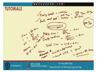
So, this is the blank page kept for the solution. So, our, so our ripping speed is 1.5 kilometer per hour. So, meter per hour, so it is coming 25 meter per minute. Empty travel speed 3.0 kilometer per hour, so 50 meters per minute. Now, let us consider what is the time required for producing or ripping a portion of 2-meter width 100 meters long.
