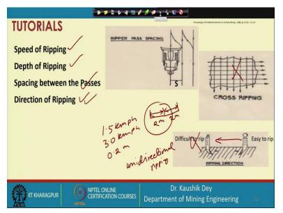
So, so far we have considered the speed of ripping is 1.5 kilometers per hour, empty travel speed is 3.0 kilometers per hour, depth of ripping is 20 centimeters which mean 0.2 meters, and spacing between the 2 passes we have not considered we have considered the width of ripping is 2 meter. So, all these widths will be simultaneously considered.
