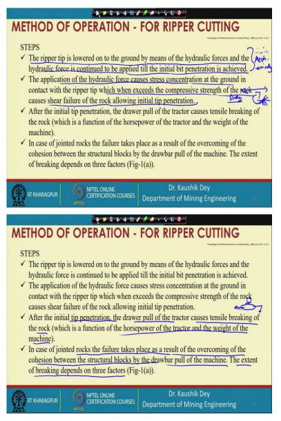
Now, if you see the steps taken by the ripper for cutting, the first job is that the ripper tip is lowered onto the ground through a hydraulic force, and the hydraulic forces continue to be applied until the initial bit penetration is achieved. If hydraulic force is not there, then you can use any mechanical force either hydraulically or mechanically, hydraulically or mechanically.
