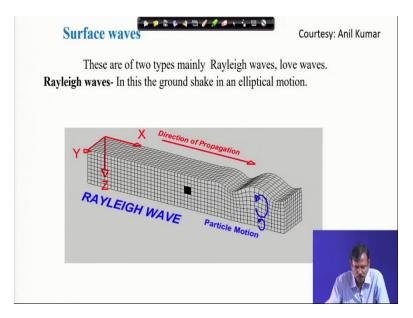
So, this is the Rayleigh wave. Propagation is almost similar to the shear wave, but it has horizontal and vertical shearing. So, this is the Rayleigh wave.
