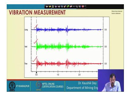
What is there in the seismograph? In the seismograph which we have seen, we have shown in the previous slide that a seismograph comprising either a magnet and coil system, if the oscillations occur to that, then the emf or voltage generated as the magnet is oscillating around a coil then emf is generating. So, when the ground is vibrating, the interest is basically oscillating, and that is generating emf. We are measuring that one.
