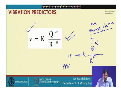
And a predictor equation is basically advised by different mining researchers where v is considered as the peak particle velocity and K is a size constant, Q is the charge quantity detonated, maximum charge quantity detonated at one instance, at one instance that is Q and R is the distance of monitoring from the blast hole. So, if you consider this one, the alpha and beta are the two power constants considered for the propagation of the wave.
