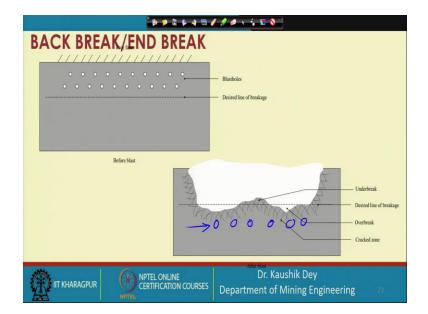
Our last result is basically the back break or end break for which we are interested. Now, let us understand what is called back break. If this is our last line of holes and we are interested in blast this portion of rock mass, we expect some additional breakages, and our final desired line of breakage may be at this position. So, we expect up to this position; for a very bad blast, we can expect up to these.
