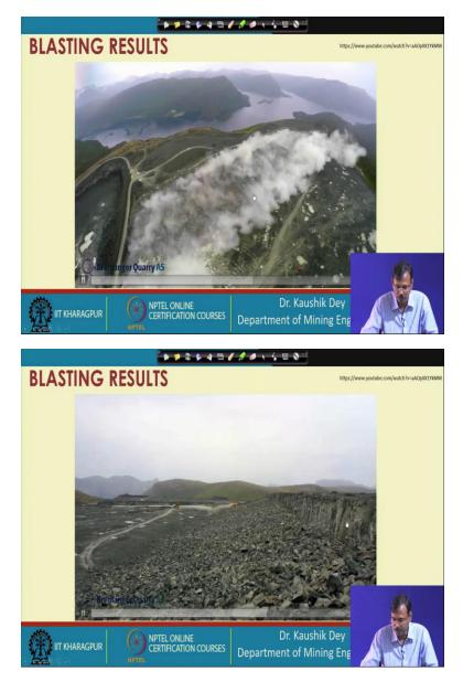
So, before that, let us look once again into the this is the largest production blast in the Norway, and you can see how this blasting is carried out. This is very well maintained 380 meter long bench is blasted here and very precisely blasted. You can see here this is a photograph taken by the drone. So, this link is available on the YouTube, and you can see the fragmented size.
