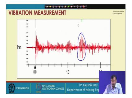
See now I have enlarged this transverse one, and this is, as this is off, let us take the blue color now. You can see when the first blast wave has arrived at this position; there is a sudden jump. So, the moment the first blast wave struck this, it started moving like this. So, this happens. Now, the particle starts moving, oscillating. You can see this is the oscillation. But as the damping is there, it is gradually trying to damp, but you can see from time to time it is again increasing.
