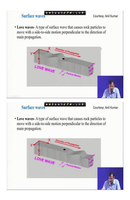
And this is the love wave. So, this is the propagation of the love wave in the horizontal direction you can see. This is the particle motions in that direction. So, these are the surfaces, and when the body waves reach the surface, only the surface waves are generated.
