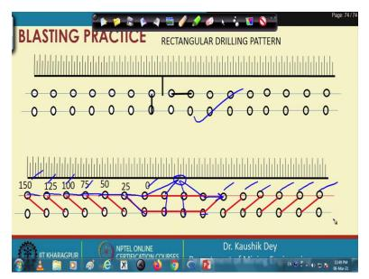
Then this is the drilling pattern, this is the drilling pattern shown here, and you can see this is the blasting pattern and this is 0 centrally placed from where this is 25-millisecond Nonel, 25-mi
