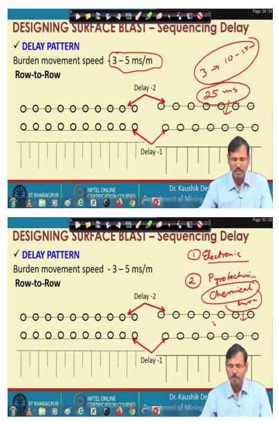
And we have discussed the delay pattern provided for blasting of the row to row and v-cut pattern. We have discussed these, and there we have considered that this delay is provided based on the burden movement, which depends on 3 to 5 milliseconds per meter of burden. So, if you have a 3-meter bench, you must consider that a 10 to 15-millisecond delay must be provided there.
