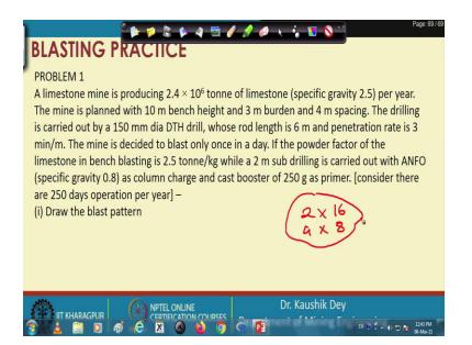
And let us solve one problem for designing a blast for actual mining conditions. Say in this problem it is given a limestone mine is producing this one with the specific gravity of this one, bench height is given, the burden is given, spacing is given, drill diameter is given, rod length, the penetration rate is given because we have considered it is from the drilling part.
