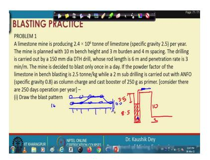
So, if l is coming 8.5 meters, then we can expect if this is our blast hole, then this is 10 meters, this is sub-drilling is 2 meters, and we are providing a charge of 8.5 meters and the stemming. Obviously, it is 3.5 meters. So, this is the section of the hole. Now, we have to provide this booster with the Nonel.
