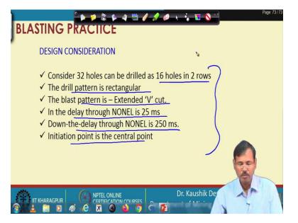
So, in consideration of that if we are considering this design criterion, if we are considering this design criterion 16 holes of 2 rows, drilling pattern is rectangular, blasting pattern is extended vcut, delay through Nonel 25 millisecond, down the hole Nonel 250 millisecond, initiation point is the central point if we are considering this.
