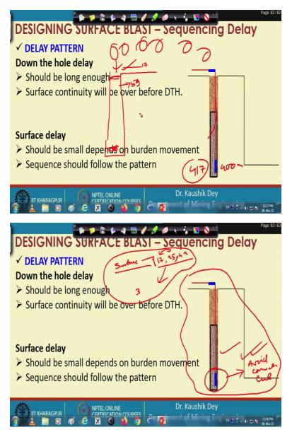
So, this will blast at 17 ms, and whatever we have drawn for that earlier one is now blasting at 42 ms, 59 ms. This is 17 ms we are blasting. This is 42 ms we are blasting. Now, what will happen in 17 ms? It will blast this portion of rock and will fly onto this. Here the charge we are providing here is 42 ms. So, this is receiving at 17, this is 42, which is why it is delivering at 59.
