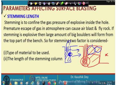
Stemming length is important because this governs the charge distribution. Suppose, to blast this rock, we need x kg, and x kg can be accommodated at this place. But what will happen in this case? This x kg is concentrated in the lower part of the rock only, and this part is completely stemmed. So, this is over stemmed, and the charge distribution is not significant.
