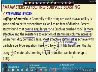
These are the criteria for the selection of the stemming material. Generally, the stemming material fragment size is considered in the range of 1 by 7 D to 1 by 25 D. This is supposed to give the best packing inside the hole. But, one very important part is that coarse angular particle is more effective. And resist the ejection of the stemming column because these have interlocking types.
