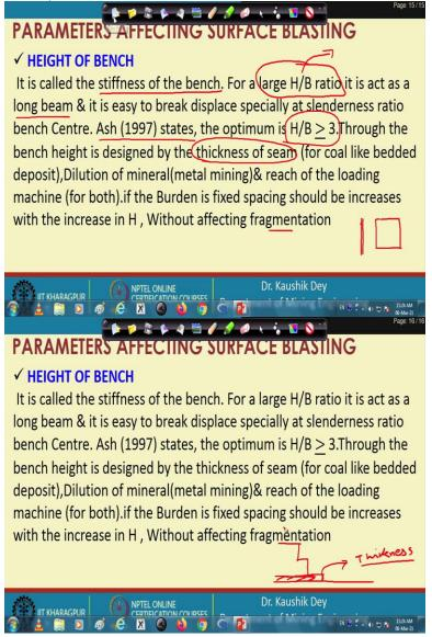
Next is the bench height; bench height dictates the stiffness of the bench. So, the H by burden ratio is considered the long beam. So, if it is creating a long beam, you can understand the long beam is very easy to break. But, if it becomes a slab like this, it is not that easy to break. So, this H by B ratio is very, very important. Ash 1997 has argued this H by B ratios should be greater than 3 for the blasting purpose.
