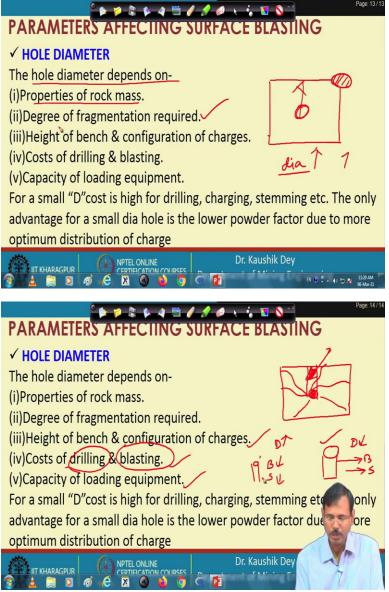
The first hole diameter is the main parameter. And most of the designing guidelines, you will find the based-on hole diameter only. So, if you see, the hole diameter depends on rock mass properties. If you have a strong rock mass, then you need to place, you need to place the explosive, more explosive for a particular cubic meter of rock. So, in that case you need to increase the diameter of the hole.
