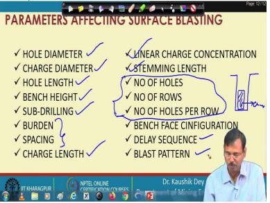
Now, let us see the least of the influencing parameters; there are a host of parameters affecting the results of the surface blasting, simultaneously the designing of the surface blast. So, these parameters are hole diameter and charge diameter. So, in our, this is the diameter of the hole, and this is the explosive charge, which is placed inside the hole in a cartridge form. So, that is the charge diameter, hole length bench height sub drilling.
