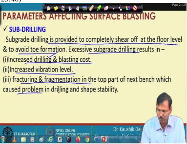
And sub drilling we have already discussed. To avoid toe formation, the sub drilling is provided to complete shear off of the floor level. But, if we go for excessive sub drilling, that may increase drilling and blasting costs because we are additionally drilling is carried out, which is unnecessary. It may increase vibration levels also. And fracturing and fragmentation in the top part of the next bench may create the problem, which we show in the next slide.
