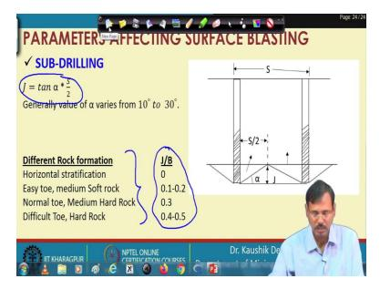
See, the fracturing that occurs at this position may create the problem. So, we sometimes go for restricting up to this only, without sub drilling, if these two are ready and readily separable. And if this part is soft, if this material is soft, we drill up to this instead of going for sub drilling.
