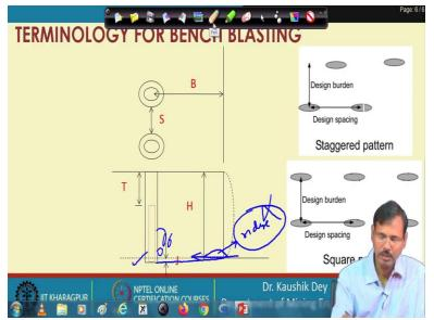
If you are looking at the hole sections, you will find out the drilled hole is, in general, a little bit longer than the bench height. If your bench height is H, then you will find out your drilled hole length is L. And this L is a little bit larger than H. So, you are basically carrying out some additional drilling, which is called J. So, this J is termed as sub drilling, sub drilling or subgrade drilling.
