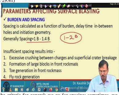
Similarly, this is the criteria for general; we go for spacing; sometimes, we may go for 1 to 2 times the burden. Also, we can go for spacing. Excessive spacing may result in crossing between the charges superficial crater breakage. So, all these other problems may arise if the spacing is
