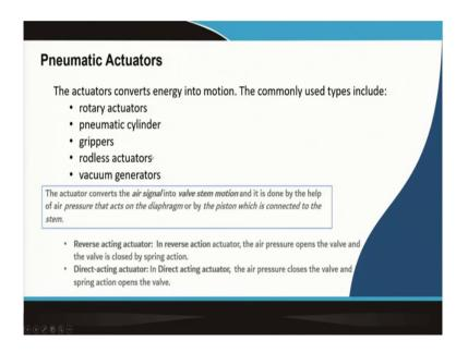
So, the pneumatic actuators that is exactly, when the valve will be allowing the your pneumatic power to go and then, do the things which will be doing the mechanical work. Now, to do that mechanical work, there could be a rotary actuator and the pneumatic cylinder, grippers, rodless actuator, vacuum generators different type of depending on the how the converts energy into motion depending on that different things are designed.
