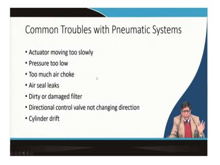
So, there will be different type of troubles in that pneumatic systems that exactly you need to know when you go to study a mining machinery. There could be the actuator moving very slowly, pressures will be too low, too much air choke, air seal will leak, dirty or damaged filter, directional control valve not changing the directions, cylindrical drift this type of problems are there.
