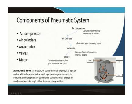
So, coming to a in a mining machinery, when you will be using a pneumatic system, the basic components which are there it will be the air compressor which will be capturing and storing the air in a compressing the volume so that this is the main job of the air compressor and then, they will have to use it.
