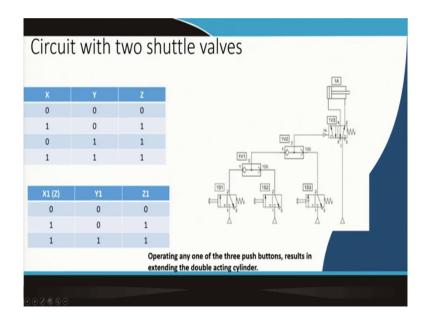
Similarly, there can be two shuttle valves coming over here. Now, you can go on developing a different type of conditions. Now, suppose you are having this shuttle valve, now you have got another shuttle valve and then, you have got a third systems you have placed over here. Now, in this case what happens? Then, if your any of this is these two are there, this or this then it will come over here.
