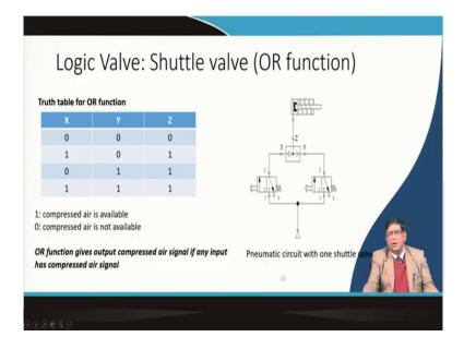
Now, the main thing is here, let us see what is that logic valve or as you have studied in your electronics that you have studied the AND gate, OR gate, NAND gate, this type of control systems with different type of logic gate can be started with the help of this valves.
