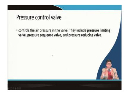
And then, the pressure control valve, it controls the pressures in the valve that they include pressure limiting valve, pressure sequence valve and pressure reducing valve.
