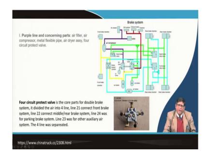
You can see also how in your dump truck the different this brake systems are there, you can have this how air compressors, you have got the front brake chambers here and you have got this rear brake chambers here. With this four, we can have a three axial vehicles. Depending on this, the circuit will be changing.
