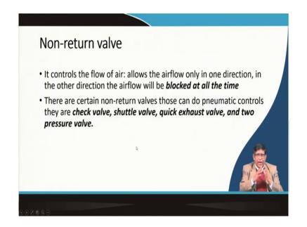
So, that is exactly the main thing used by the direction control valve, but there to give the operations in a proper way, you will have to see that the air does not come back to or does not return. So, sometimes, it will have to move all the time in one-way so, there you will be using this non-return valve where the flow of air they are allowing, the air flow only in one direction, in the other direction the airflow will be blocked at all the time.
