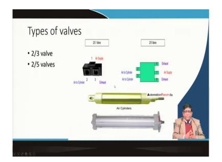
So, these valves they are exactly used say you can see that when we say a 2 by 3 valve means we have got air, exactly supply is coming, and we have got these two exhaust that is air will be going to the cylinder. Similarly, a 2 by 5 valve that is your we are having air to cylinder coming by these two ports and then, it has got exhaust and the supply. So, all these things they will be inside a cylinder, how the air will be entered into, they will be given by different valves.
